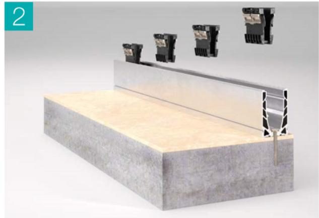
Lay the clamps inside the profile every 10". Do not place the clamps on top of the anchor screw.
