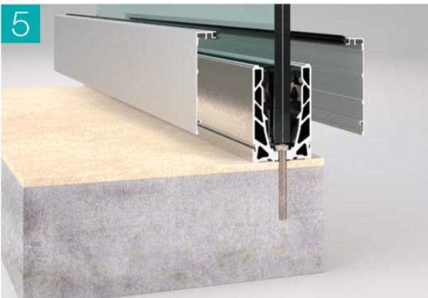
Snap the cladding in place, to which the seal has been previously inserted.
