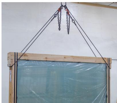
For wood cases handling using a 10,000 lbs forklift boom or 3 Ton overhead crane. Adjustable for 48" x 84" up to 96" x 144" cases.
