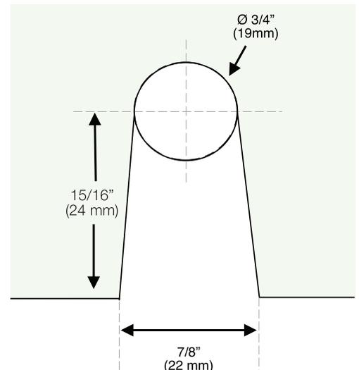
Cut-out used when fixing glass panel to wall or floor.
