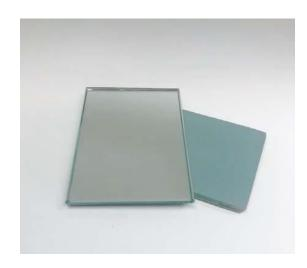
Copper-free mirror is made by thoroughly cleaning annealed glass and sensitizing it with a diluted solution oft in chloride. Silver nitrate is sprayed onto the surface of the glass along with other proprietary chemical configurations. After silvering, a two-coat paint system is applied to encapsulate the formula with low-lead or lead-free solution along with a copper-free paint solution.
