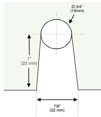
Cut-out used when fixing glass panel to wall or floor.
