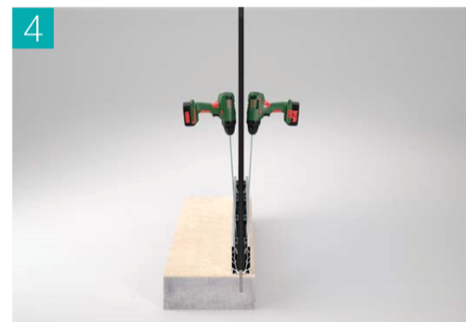
4 Adjust the inclination of the glass using the screws on the clamps with a 5/32" (4 mm) hex driver and tighten.
