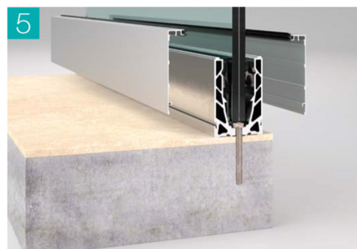
5 Snap the cladding in place, to which the seal has been previously inserted.
