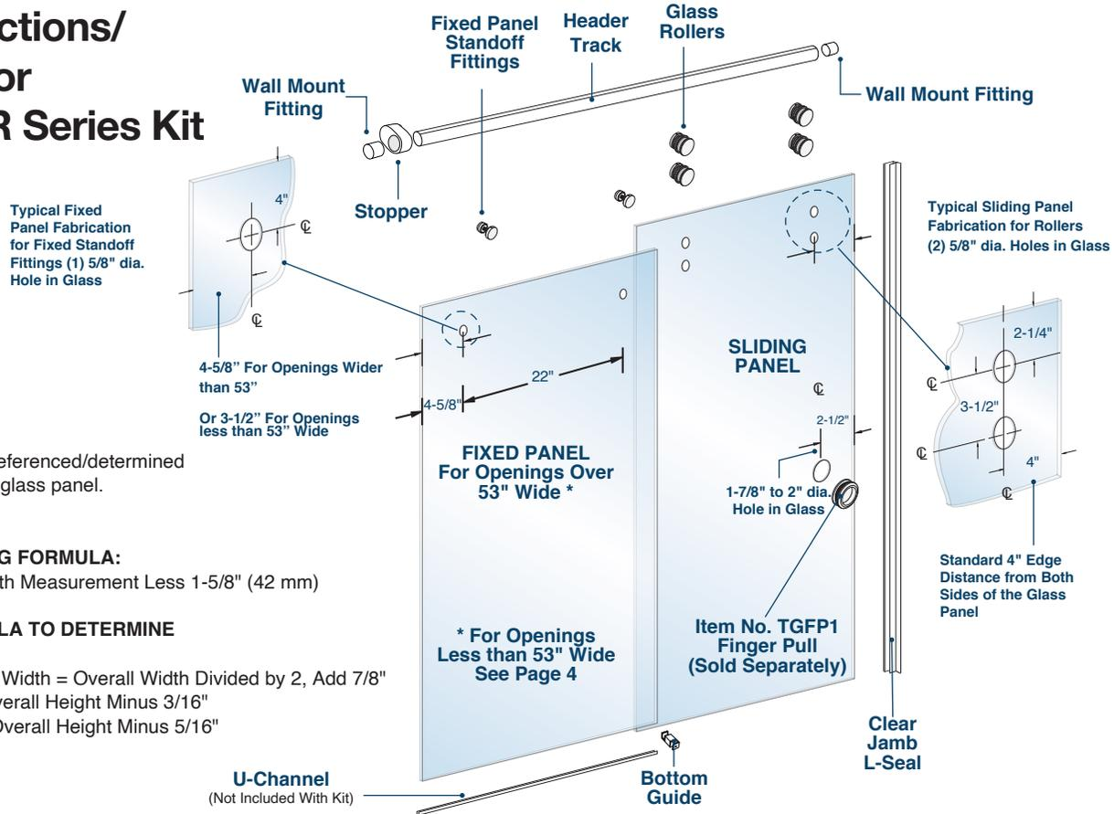
**NOTE:** The Overall Height is referenced/determined from top of curb to top of fixed glass panel.
